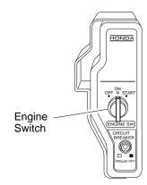
Figure 18 - Engine Switch
